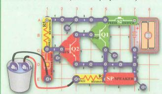
If the two loose jumpers are placed into a cup of water, an alarm sounds. You could put this circuit in your basement and use it to alarm you if the basement floods during a storm. If you slowly add salt to the water, you will hear the pitch slowly increase.
