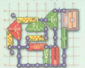
This is another adjustable oscillator circuit, which also includes an LED. Although the LED appears to be on, it is flashing at a very fast rate. The  $0.02\mu F$  or  $0.1\mu F$  capacitors can be placed on top of the whistle chip to lower the frequency. The  $10\mu F$  may also be placed there, but then the frequency is so low that the LED is flashing and the series of clicks is heard. The speaker may be replaced by the 2.5V lamp.
