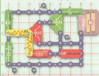
This circuit is an oscillator controlled by a discharging capacitor. Turn on the slide switch and press the press switch. The sound is loud but slowly goes away.
